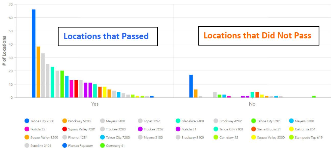
**Figure 6. Pole clearance (8ft-Conductor) Results by Circuit**
